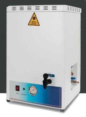
Water supplied from the distiller is boiled and evaporated with the help of resistances inside the device. With the condensation process following evaporation, the water is purified from salt, minerals and various metals and pure water is obtained.
