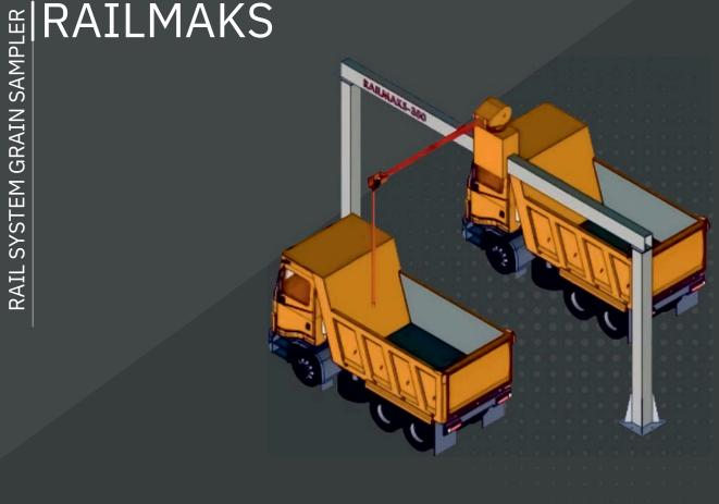
Railmaks sampling probe is designed to take a representative sample of grains such as wheat, barley, rice, rye, corn, beans and chickpeas from any open-top vehicle. The telescopic arm mounted on the movable rail system can move forward-backward, up-down and right-left in a circular motion thanks to the hydraulic system. Depending on the turbine power, it carries grains from a distance of up to 50 meters to the laboratory in as little as 10 seconds.
