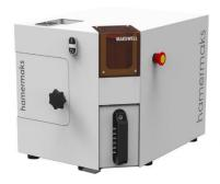
If whole wheat is to be used in falling number analysis (FN meal), the wheat must be ground and turned into powder. The wheat must be ground with a standard and correct method, otherwise deviations will occur in the falling number values. For this, hammer mill (Hamermaks) devices produced by Makswell in accordance with the standards must be used. The wheat ground in the Hamermaks device is passed through a 0.8 mm sieve to obtain a homogeneous sample.
